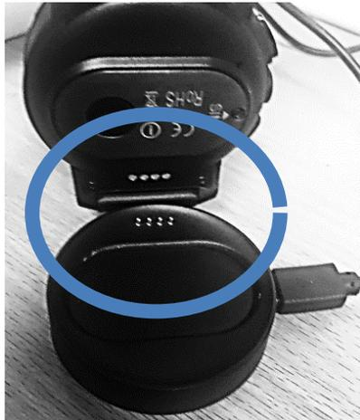
2. Place the watch on top of the round recharger base making sure to connect the recharge pins on the bottom of the watch with the 4 pins on the magnetic recharge base
